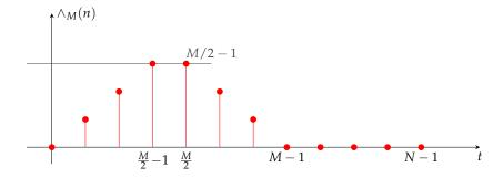
**Figure 2.** Unit energy triangular pulse of length  $T_0 = MT_s$  and duration  $T = NT_s$ . The signal is smoother, i.e., changes more slowly, than the square pulse of equivalent length.
