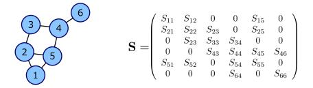
**Figure 1.** Example of a six node graph and its corresponding graph shift operator. Observe that the nodes are labeled, and that the graph shift operator is nonzero only where there is an edge, or in the diagonal.
